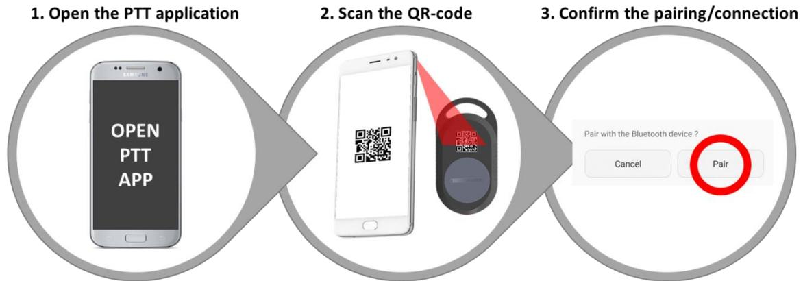
As an app developer, you will need to implement a QR-scanner into your application. Within the Android operating system this can be made using Google's mobile vision API, or for iOS using iOS' AVFoundation framework (more on this in section 5).
