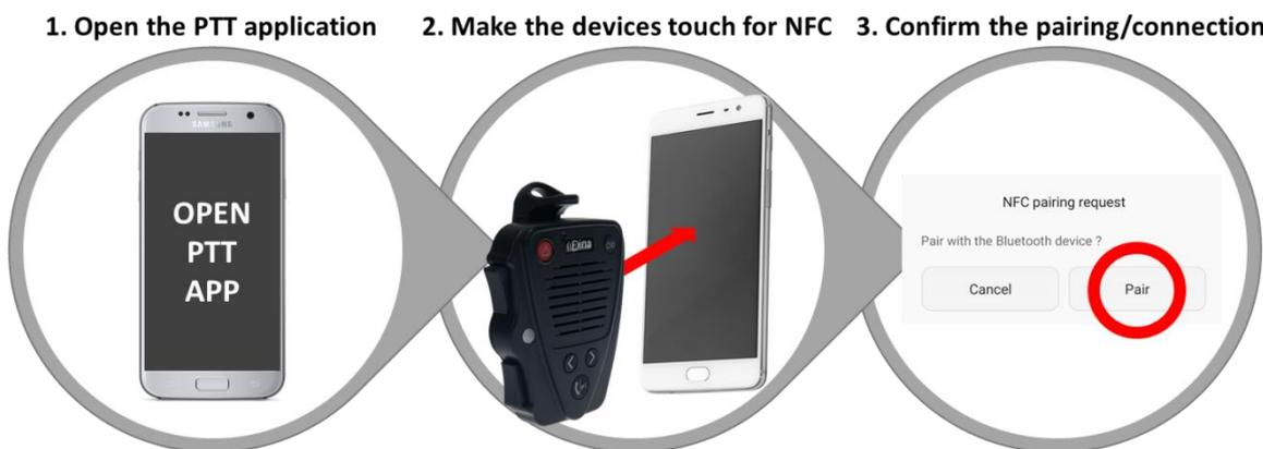
As an app developer, you will need to add the necessary functionality to the application so it can read our NFC tag. This can be made by using Android’s NFC API (more on this in section 4).
